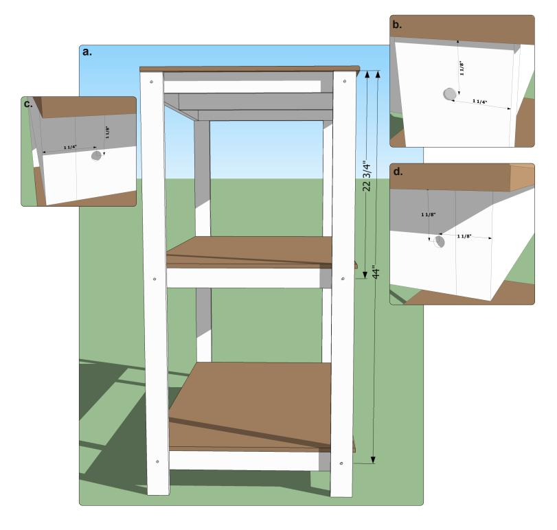
The bolt-hole locations along the legs can be seen in Figure (a) and Figure (b) and are identical for the front and back legs. The bolt-hole locations on the frames are shown in Figure (c) and (d). Note that the holes along the front of the frames are 1/8" closer to the front which results in the front legs extending 1/8" forward for a slight shadow line and fully hides the rough edges at the ends
